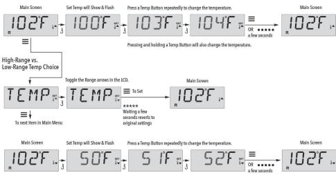
Pressing and holding a Temp Button will also change the temperature.
