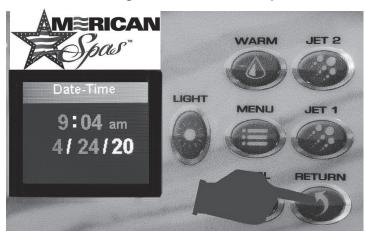
Once the screen has reverted back to temperature, you can now adjust Filter Cycles. **NOTE: You do not necessarily have to adjust the Filter Cycles because the default factory settings give you two Filter Cycles per day automatically.** In any case, to access the Filter Cycles, press the MENU button.
