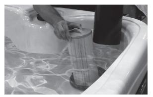
Unscrew the cartridge and remove it.
